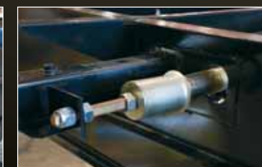
3" slide rams with electric motor
