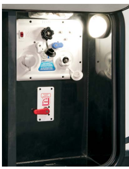
Central Convenience Center, which includes an outside shower, black tank flush, winterization system, cable and satellite hookups and battery disconnect, all in a well-lit area.
