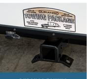
**DURANGO TOWING** PACKAGE 3,000 LB tow rating, 300 LB hitch rating.
