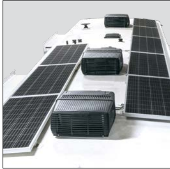
(8) 220W solar panels = 1,760 Watts of solar power
