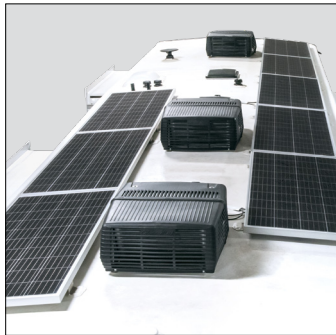
(8) 220W solar panels = 1,760 Watts of solar power
