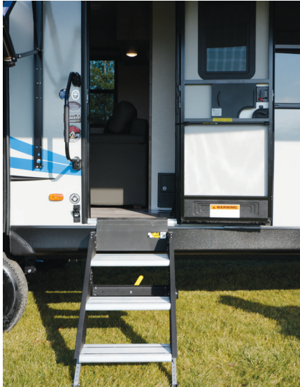
The Lippert Components Solid Step folding entry step system is easy to deploy, and adjusts to uneven campsite terrain.
